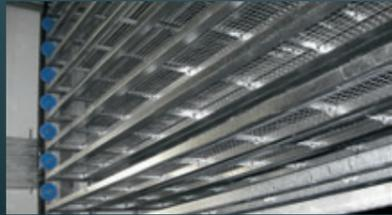
Different shelf sizes and a storage system that is variable in terms of the number of stacked levels and the number of shelves in a row allows a modular system design according to the required freezing capacity and number of storage locations as well as the overall dimension.
