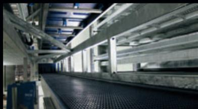
The products are moved on the shelves in a manner that is gentle to the packaging and provides you with considerable freedom in the selection of package sizes and package types. You can therefore simultaneously cool or freeze products in cartons, in trays, or in plastic containers (e.g. E1, E2, or E3) in a single system.
